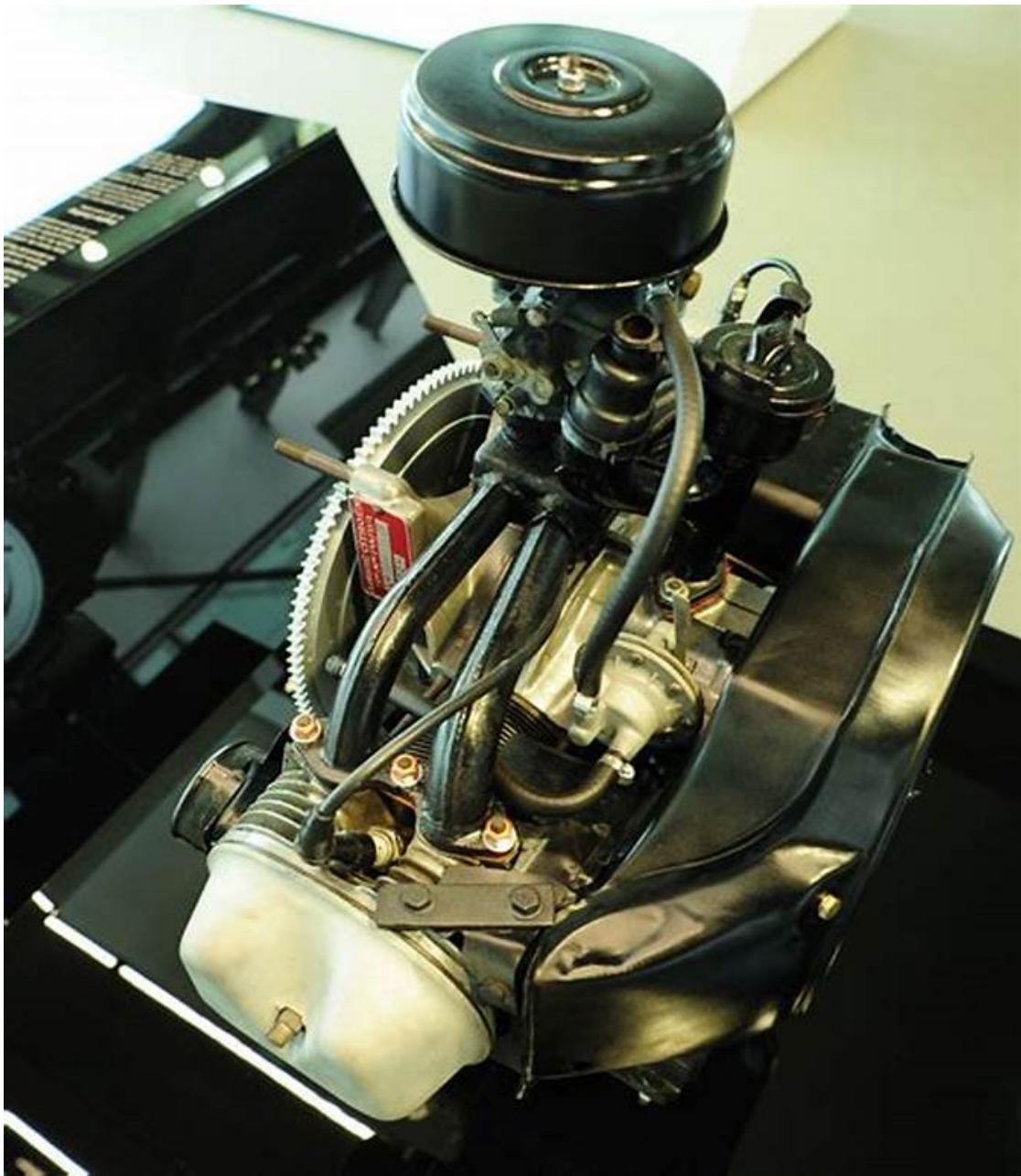
The 2CV's air-cooled engine, a marvel of simplicity and efficiency.
