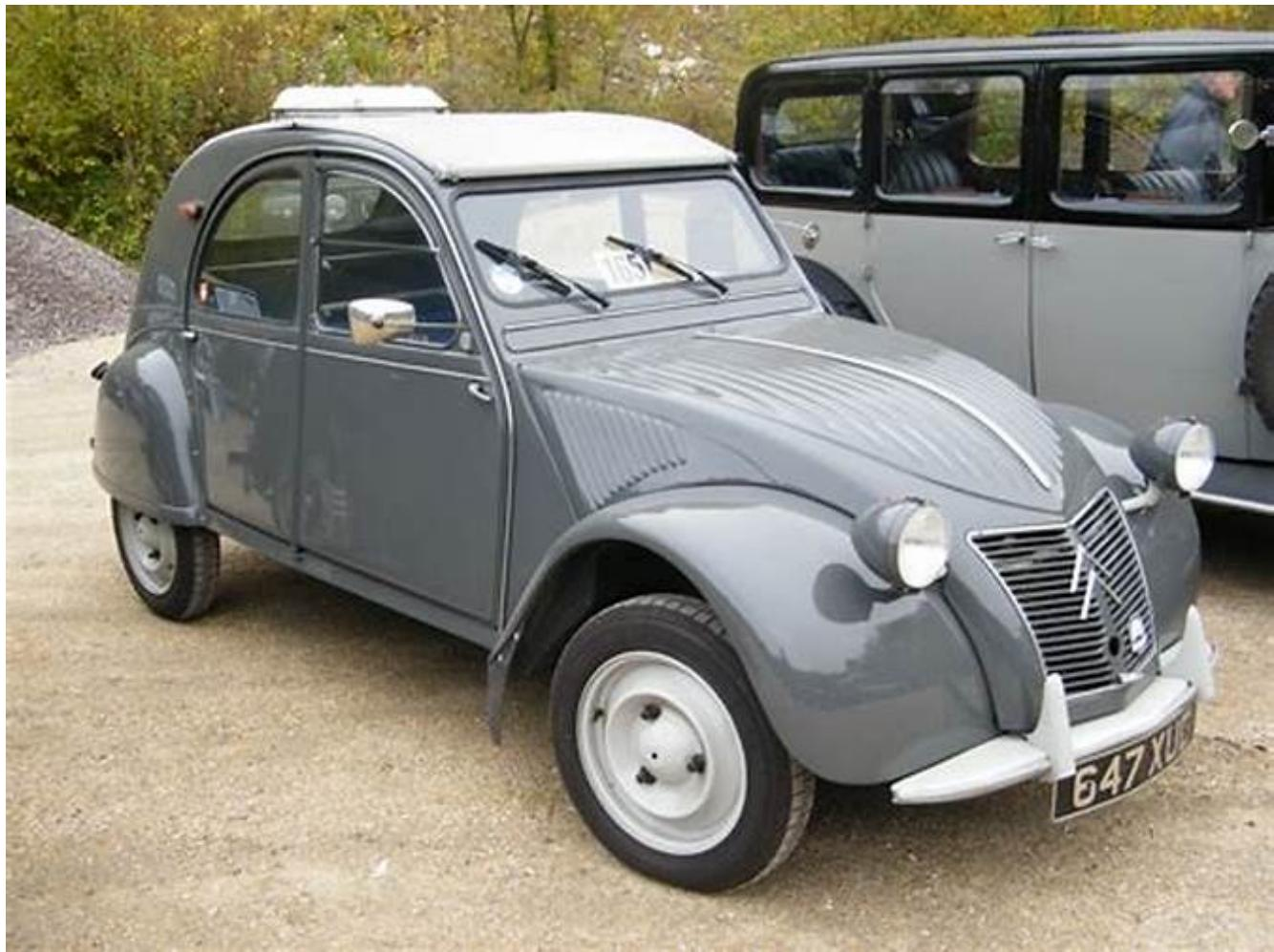
The 2CV's design was a radical departure from the automotive norms of the time. Its unconventional appearance, featuring a corrugated body, canvas roof, and minimalist interior, earned it the affectionate nickname "the ugly duckling." However, beneath its quirky exterior lay a surprisingly capable and versatile machine.
